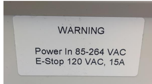
Fig 2.4 AC Voltage E-Stop
